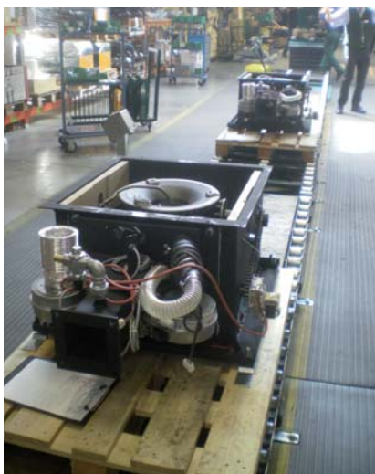
The heaters are assembled in two stages. Stage 1 results in a module, stage 2 is the finishing touch.
